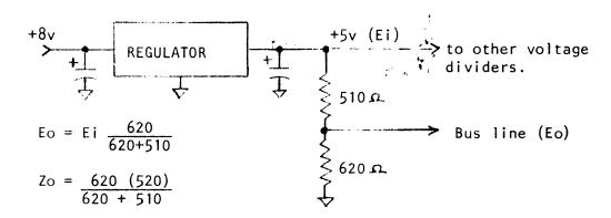
The effective output voltage to each bus line is >2.7 volts. The impedance of this termination is about 275 ohms.
