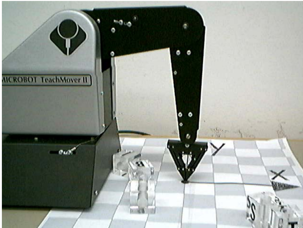
The Robot In Its Home Position (The size of each square on the floor is 50mm)
