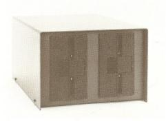
The 5½" MDX dual drive cabinet will mount two Shugart SA-400's or two Micropolis drives. It includes a 5" fan, & 5VDC @ 3 amp and 12 VDC @ 3.4 amp power supplies. The steel cabinet is dual tone blue and grey to match the I-8080 series enclosures.
