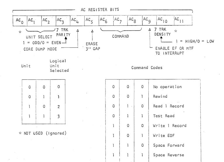
The "000 command" will cause an "illegal command" error (set EF and cause an interrupt) if an MTGO instruction is executed while this code is present in the command register. However the unit is selected when the command register is loaded regardless of command.
