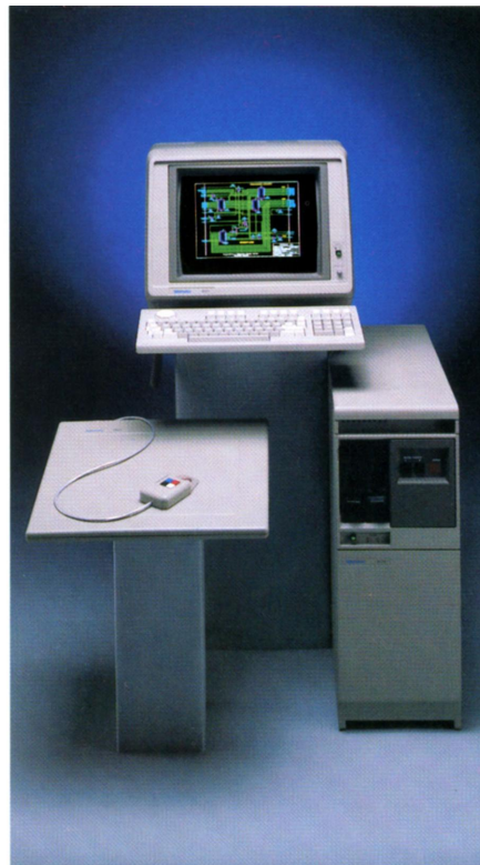
Figure 10. Another configuration could include a Tektronix color raster 4107 or a 4109 Computer Display Terminal paired with the Tek 4170 Local Graphics Processing Unit and the 4957 Graphics Tablet.
