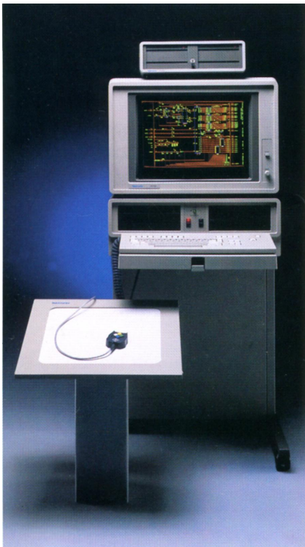
Figure 9. One PLOT 10 TekniCAD configuration could include a high performance terminal, such as the 4115B.
